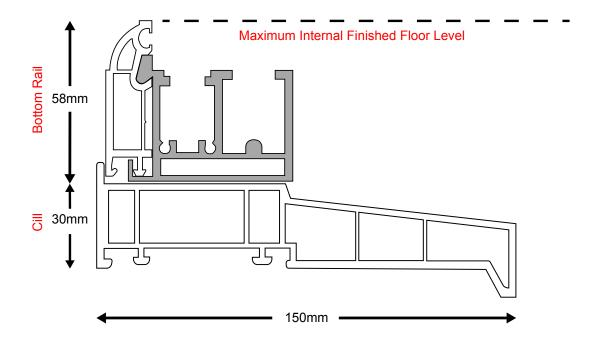
The enclosed PVC New Wave Door threshold section (pictured above) is to help you achieve the correct internal floor level and should be used as a template.
