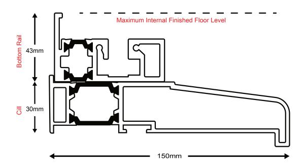
The enclosed Aluminium New Wave Door threshold section (pictured above) is to help you achieve the correct internal floor level and should be used as a template.
